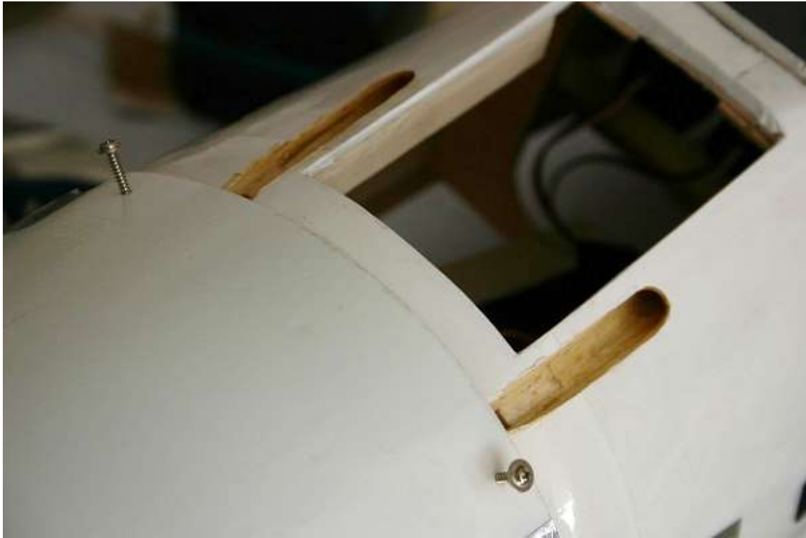
Battery access hatch and gun recesses
