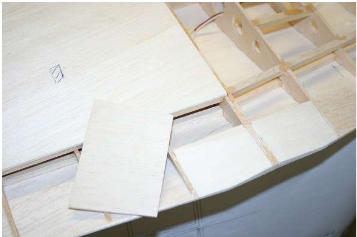
Wing bolt reinforcement fitted and then over sheeted
