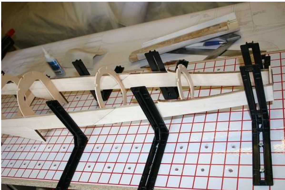
Use SLEC building jig to allow formers to be added
