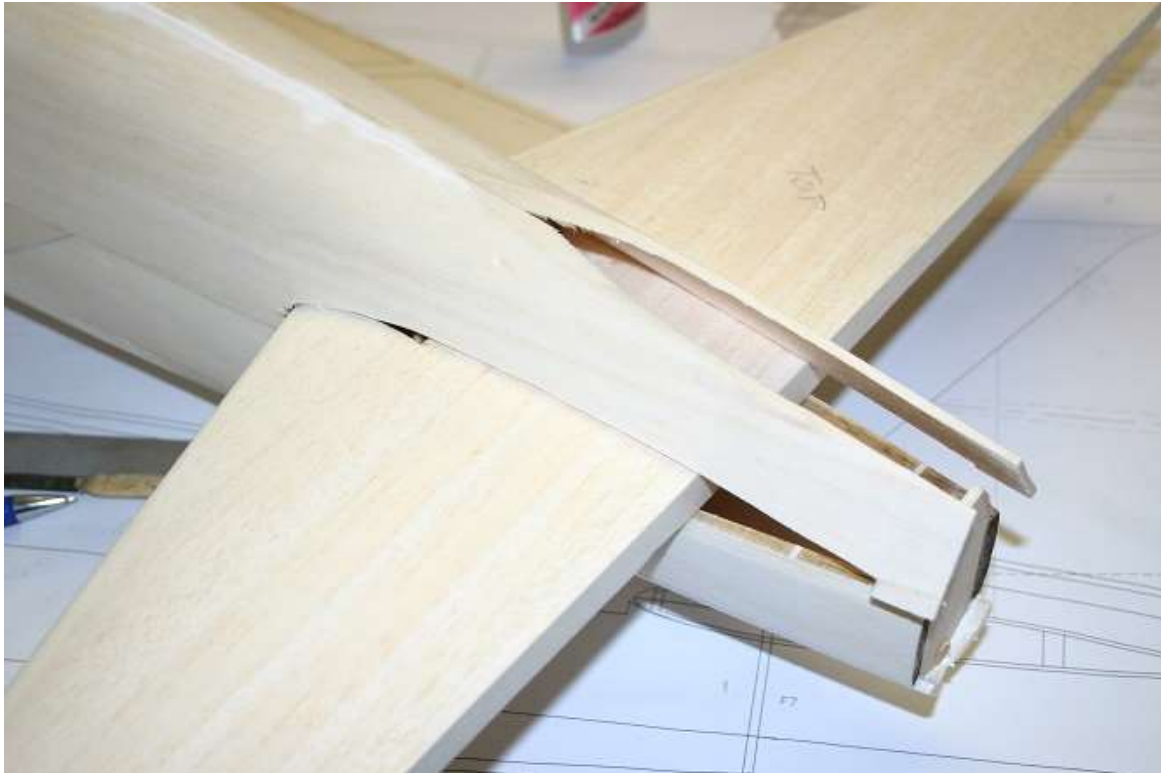
Correctly positioned tailplane. Re-glue the fuselage edges against F8
