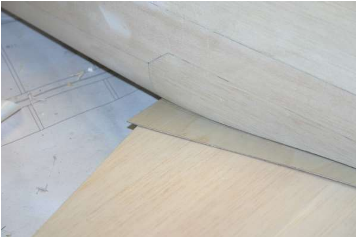
Fit the wing then slide the cut ply fairing into position
