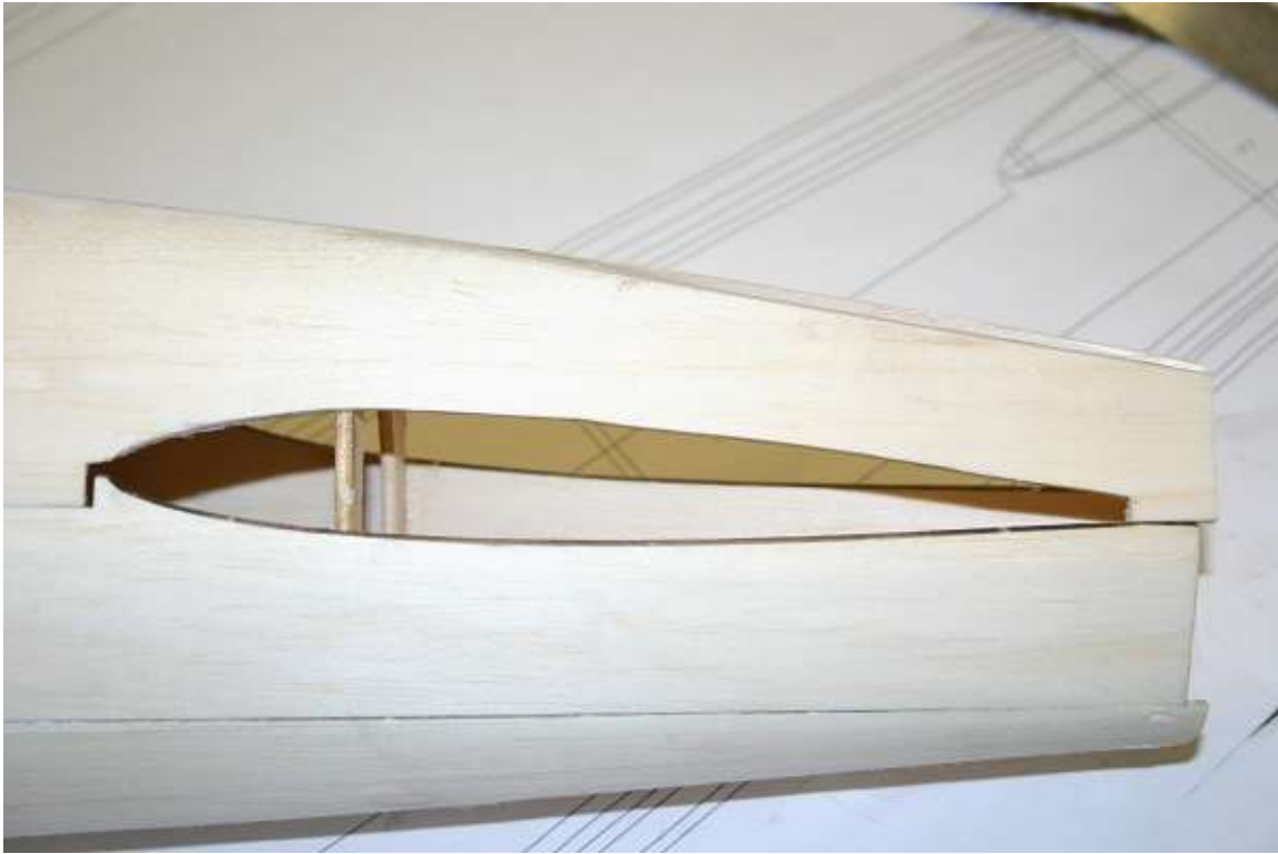
Sand the top of the fuselage flush to reveal the fin opening
