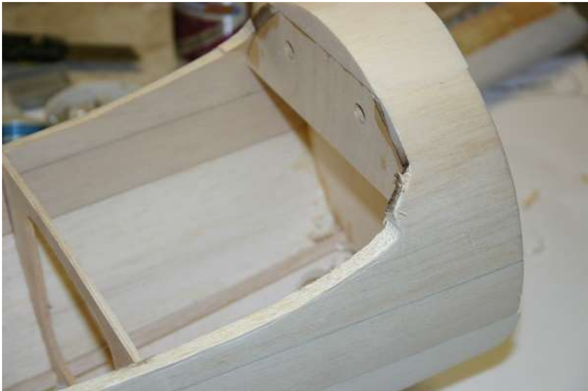
Trim fuselage wing seating to match wing angle
