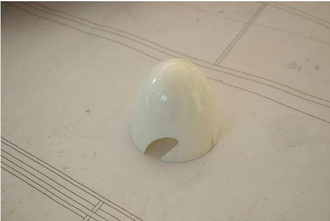
Plastic spinner trimmed to suit 3-bladed prop
