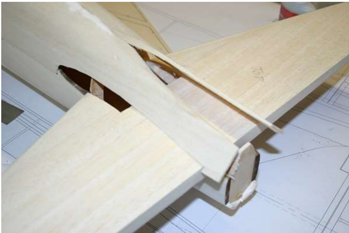
Break open the fuselage against F8 to allow the finished tailplane to slot through
