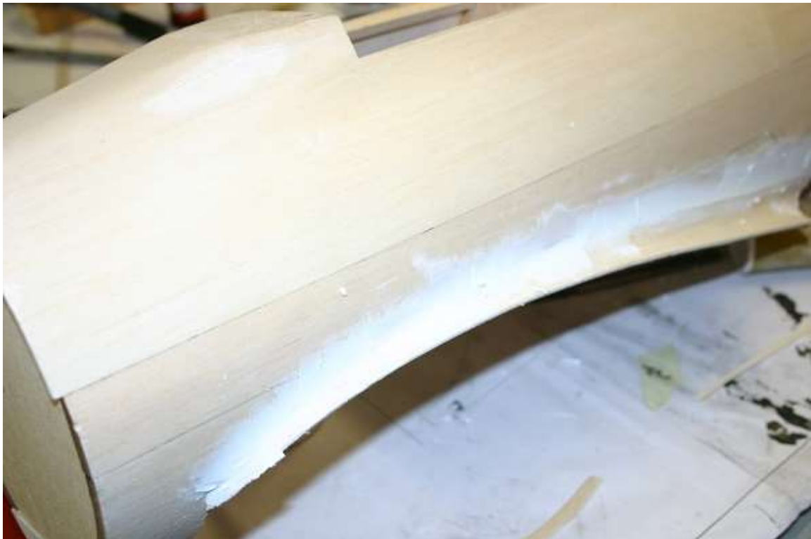
Lightweight filler to blend smoothly into fuselage
