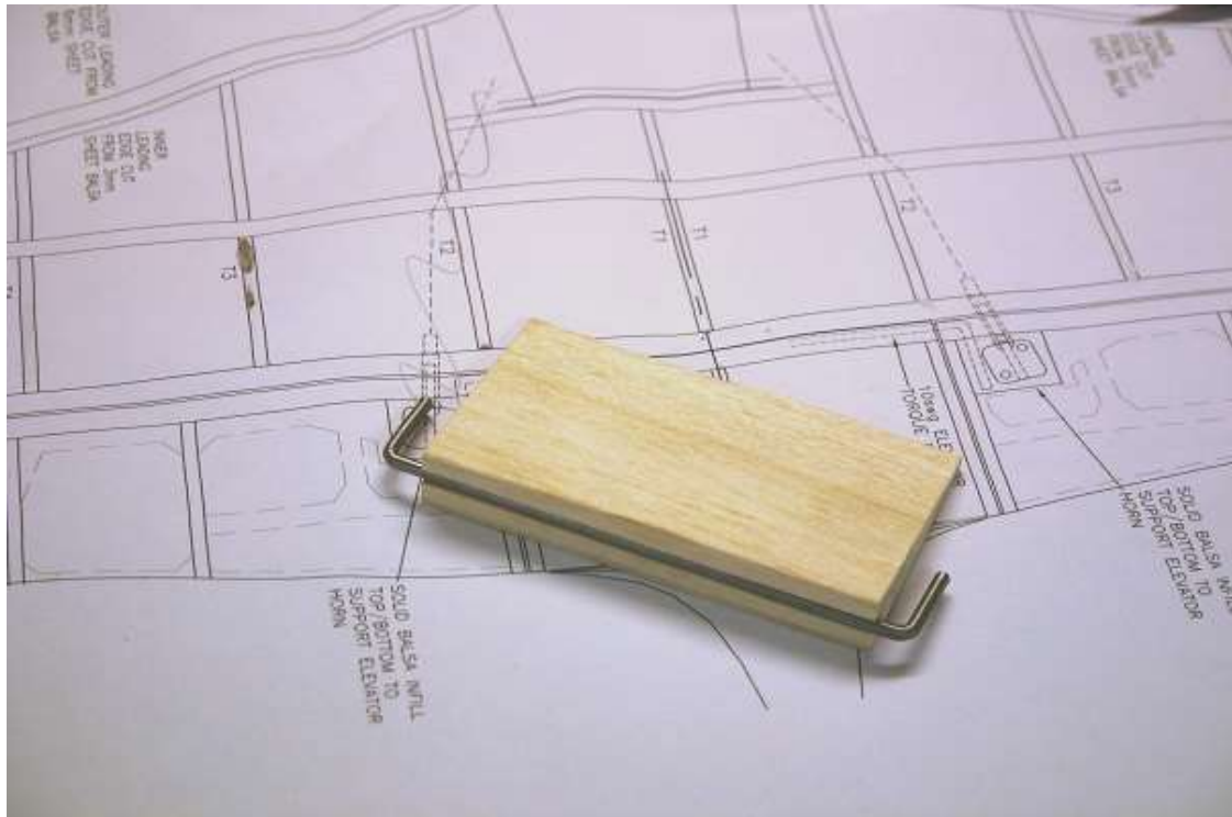
Channel a slot and add the elevator torque rod
