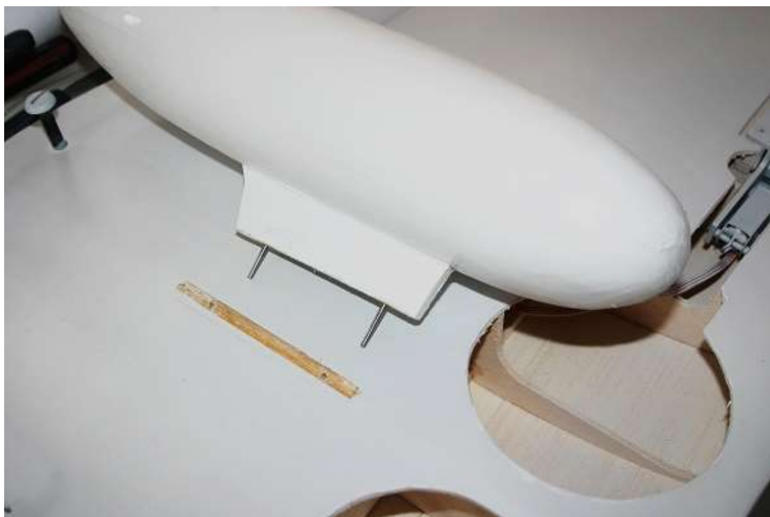
Drop tank shaped from solid balsa
