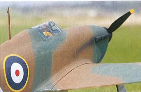
rods and the remainder of the onboard radio gear. Both versions (i.c. and electric) will need ballast in the cowl, which should be placed as far forward as possible. The prototype needed just over 10oz (283g) of lead to balance at the C of G, providing the model with an AUW of 8 lb 4oz (3.7kg).
