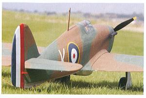
Early Hurricanes flew with twoblade props so it's one aeroplane that seems to be able to get away with a normal model flying twoblader.
