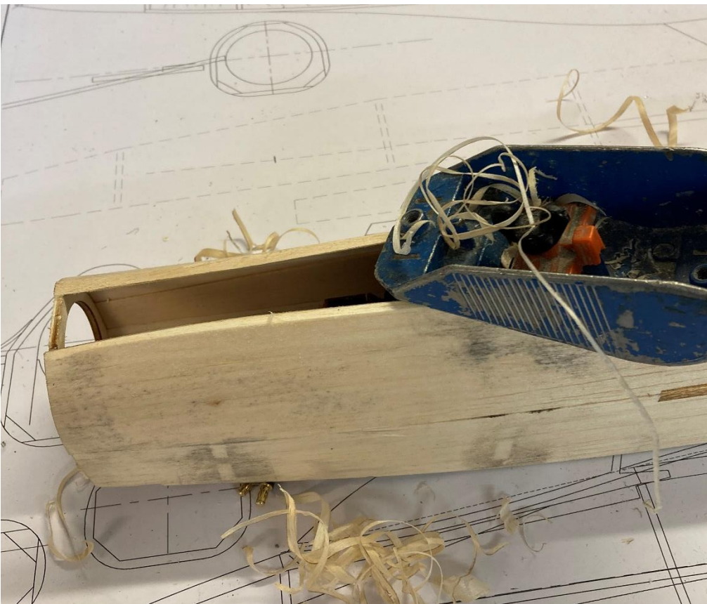
Remove excess overhang to the top of the formers. Note step at the rear-see plan
