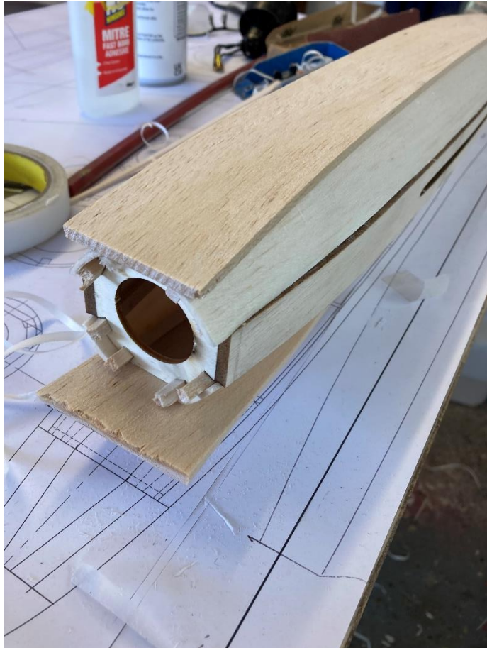
Sheet the top and bottom of the fuselage with 5mm soft balsa
