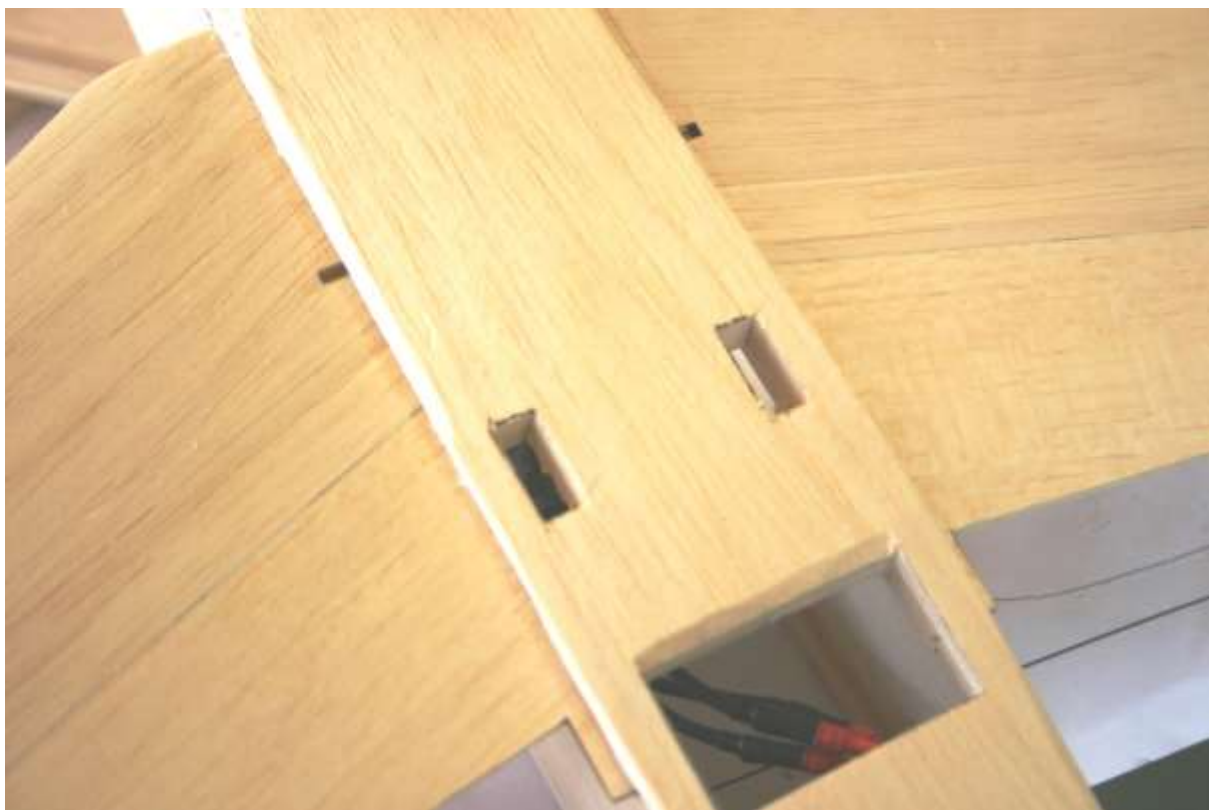
Cut openings for aileron servos
