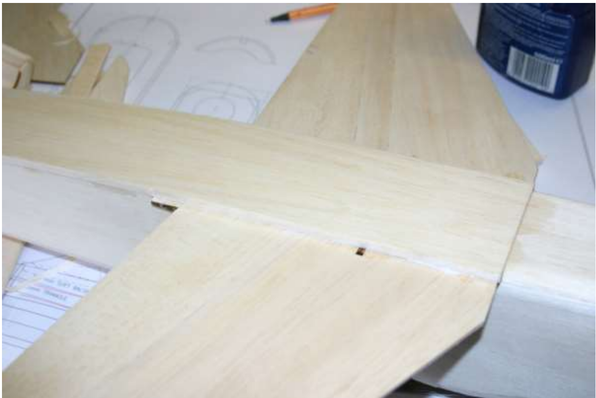
Sheet the rear underside
