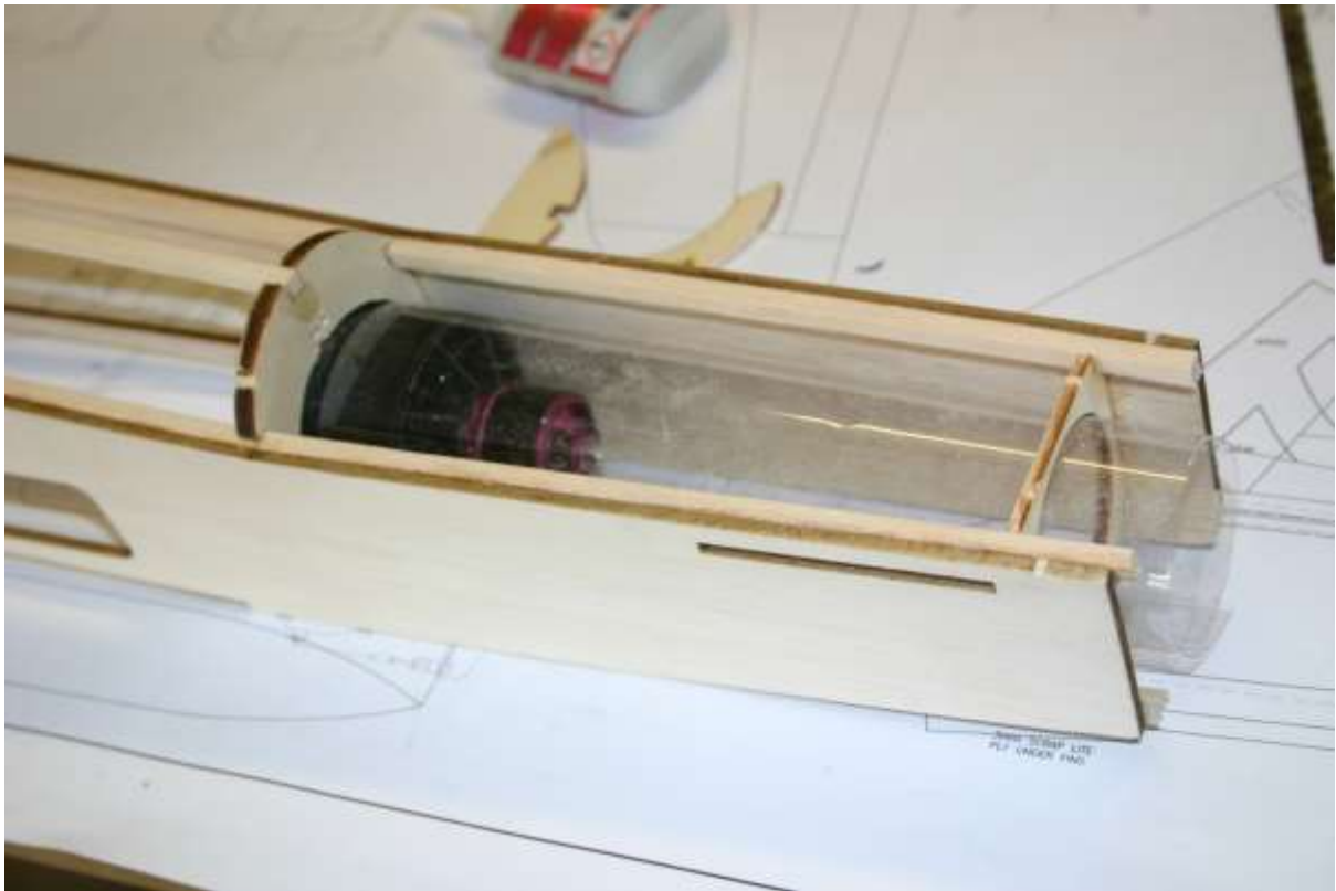
Add former 10 and make up the thrust tube
