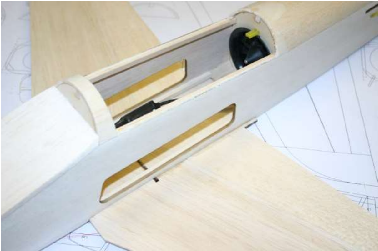
Add wing doubler 13 and glue the wings on to fuselage
