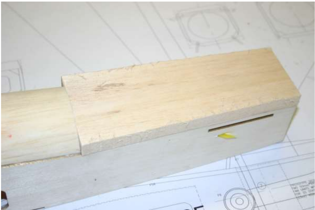
Add the rear fuselage 12mm sheeting
