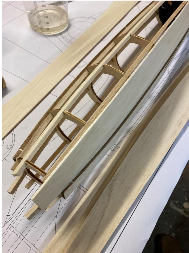
Sheet the top and bottom sections of the fuselage, using soft and wetted 2.4mm balsa
