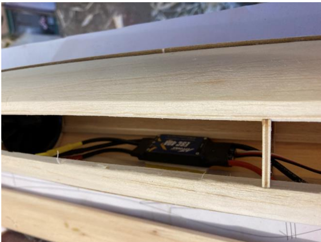
Fit and test the ESC and secure this into the model. Note that ESC timing should be set to high
