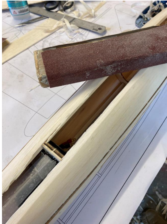
Using a sanding block, sand the top and bottom edge of the 2.4mm sheeting, back to the stringers and the top/bottom edges of the formers
