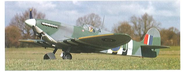
To improve the ground handling the undercarriage has been cranked forward slightly, although to the untrained eye the effect is barely noticeable.
