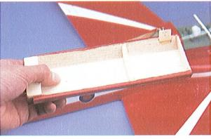
The hatch is cut after fuselage assembly has taken place.
