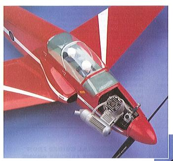
engines and 3-channel radio operating ailerons, elevator and throttle. The construction is very similar to that of the small electric Spitfire and Me109 'Dogfight Double' produced as a free plan a couple of years ago.
