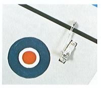
Wing mounted aileron servos have worked well for me in the past, as they have here.
