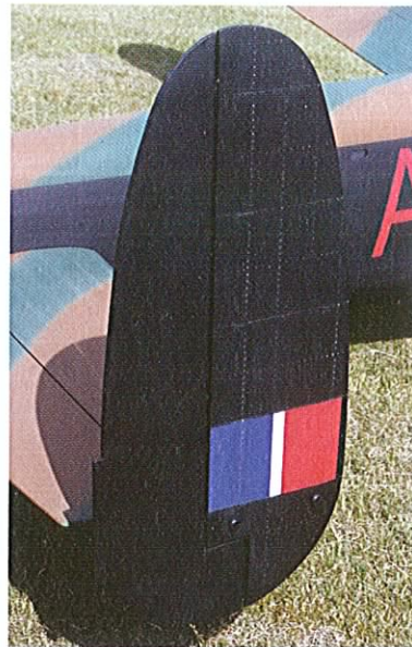
The Lanc' breaks down into nine parts for transportation and storage - three of these comprise the tailplane which has detachable fins.
