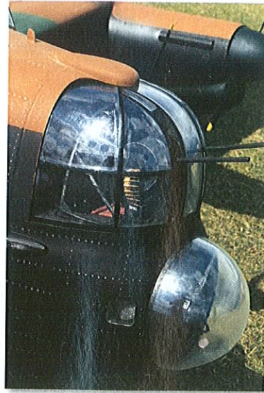
A whole selection of household items were used to fit out the turrets. The bullet belt, for example, is made using cut down cocktail sticks and self-adhesive tape.
