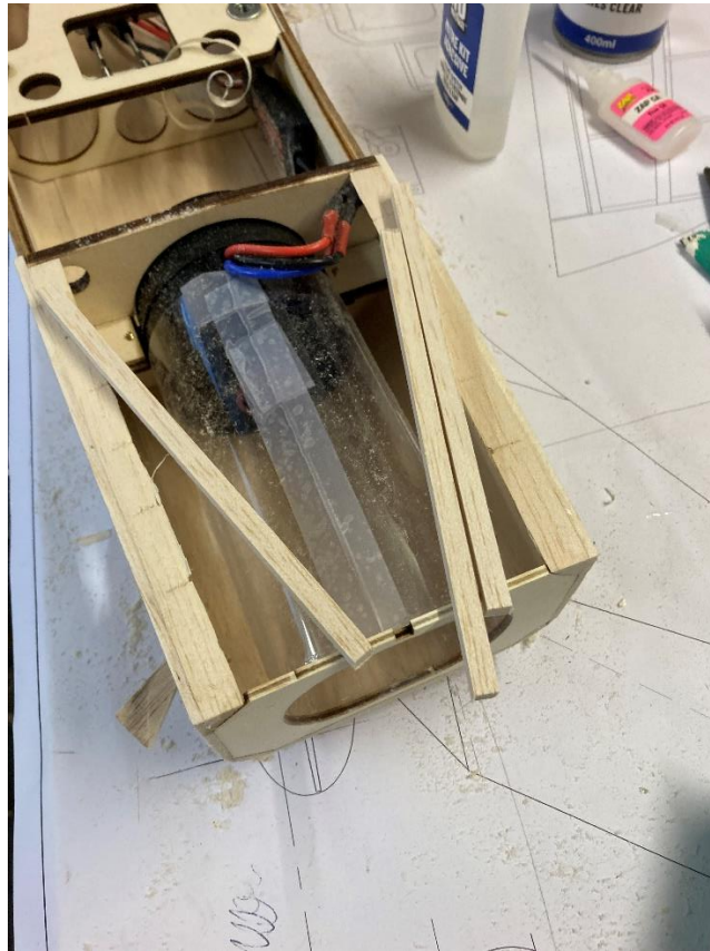
Tailplane slot strengthener
