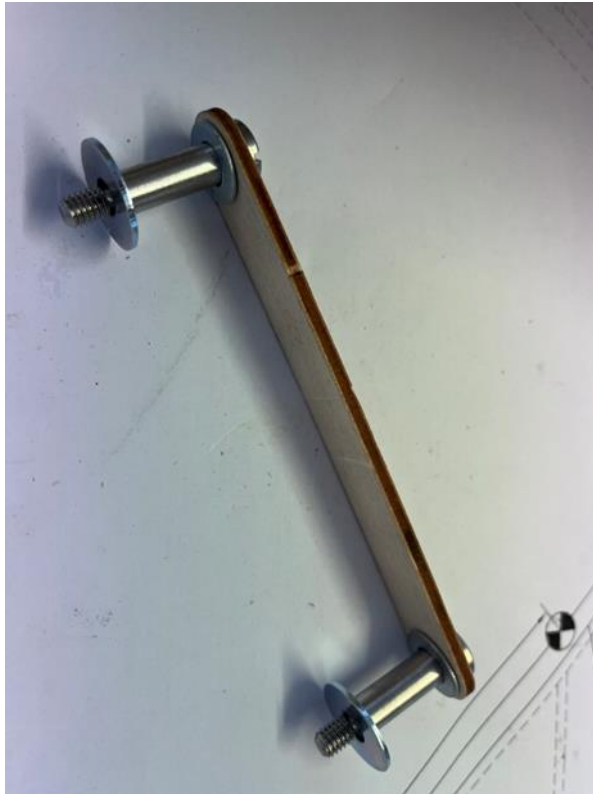
Make up the top cross bar
