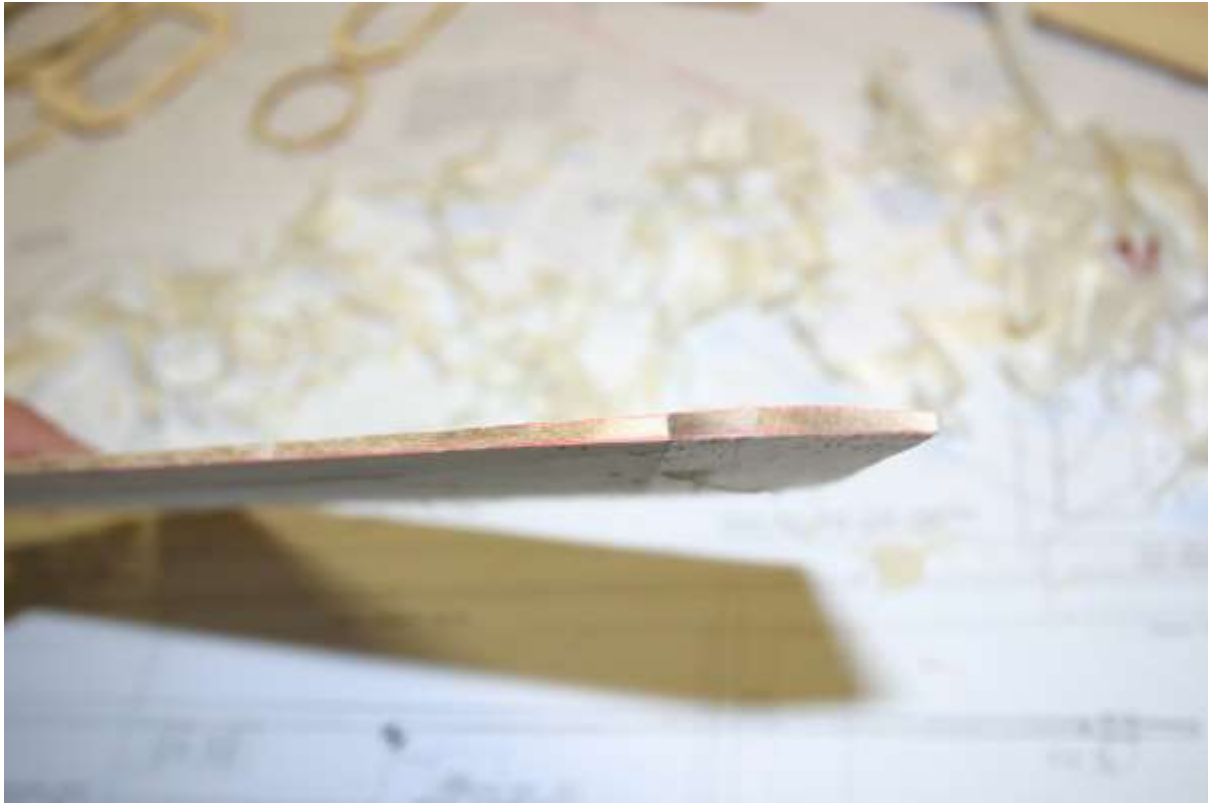
Edge mark indicating depth of material removal
